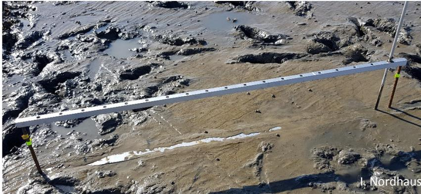
Sedimentation erosion bar (SEB)
